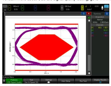
Figure 44. USB 2.0 Hi-speed near-end eye pattern test.
