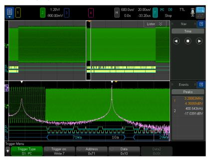
Figure 37b. Gated FFT time correlating the FSK frequency hopping with an I2C command (write 7 at 0x71 data 10).
