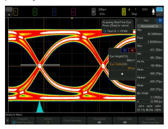
**Figure 20.** A real-time eye diagram measurement of a clean 1-Gbps PRBS embedded clock signal. The histogram measured about 22-ps rms jitter.
