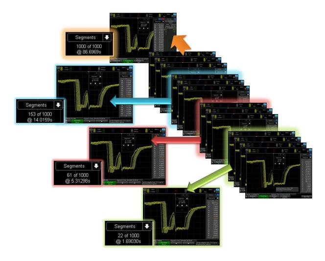
Figure 22. Segmented memory graphical representation.
