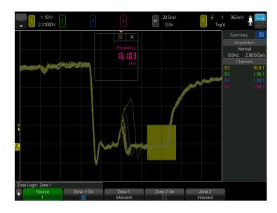
Figure 12. Hardware zone triggers immediately.
