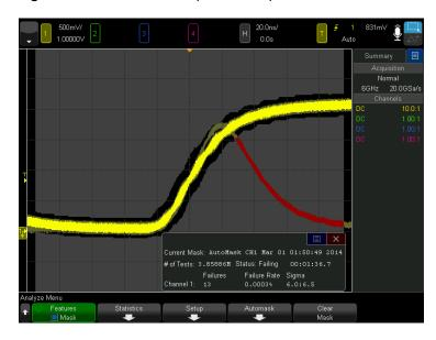
Figure 40. Limit testing of infrequent glitch.
