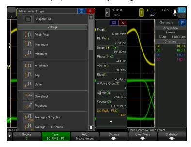
Figure 50. Measurement selection menu. Swipe and double touch to select.
