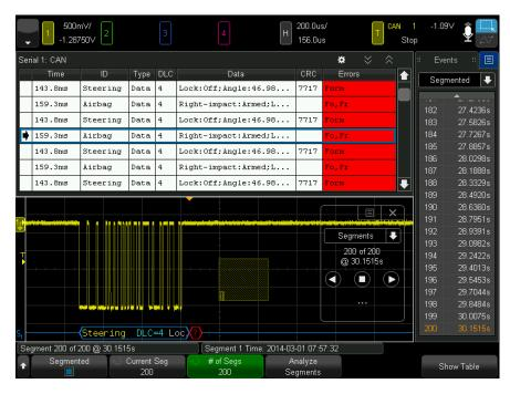
**Figure 25.** Segmented memory + serial bus decode + zone trigger.
