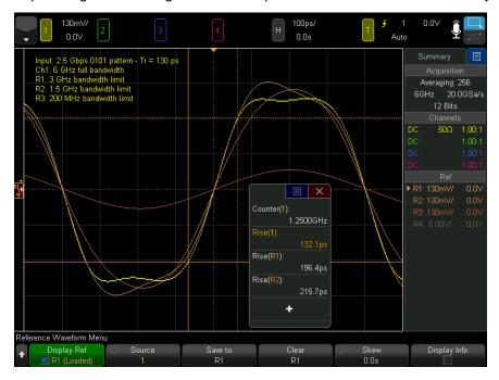
Figure 1. Measuring the rise time of a 130-ps rise-time edge (10 to 90%). The rise time measurement by
