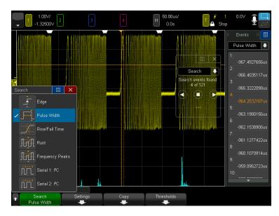
Figure 42. Searching for and navigating to a specific pulse width.
