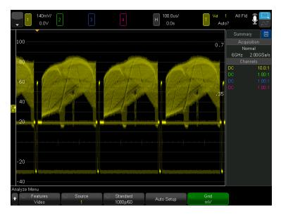
Figure 45. Triggering on a 1080p/60 signal.
