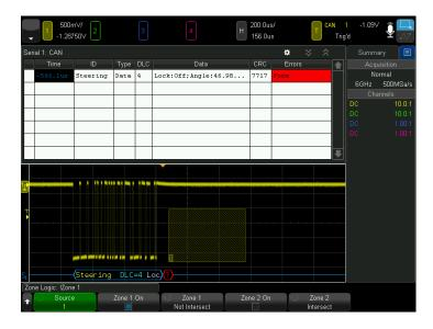
Figure 14. Now you have isolated steering errors from all other CAN bus errors.
