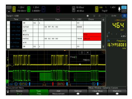
Figure 30. USB 2.0 protocol trigger and decode option display.
