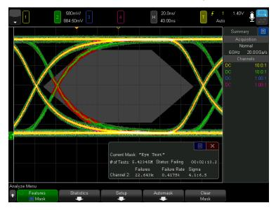
Figure 41. Mask testing of serial data.
